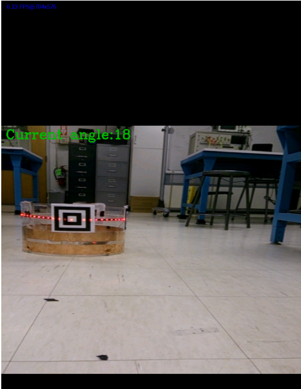
Figure 8: Screenshot of bot's vision through the periscope. Bot recognizes station is 18° from center.
